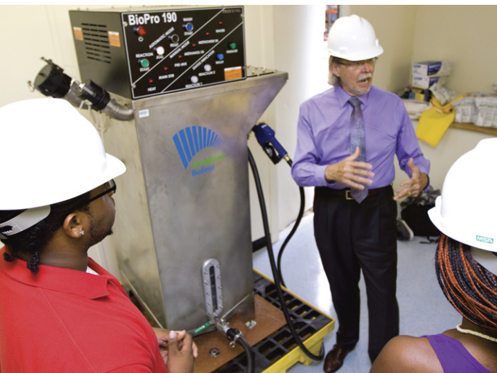
Jay Matteson demonstrates the College's biodiesel processor, which turns leftover cooking oil (yellow grease) into biofuel.
