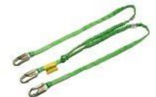
Double-legged lanyards are used for 100% tie-off safety. It is important, however, to understand the safe and proper use of a double-legged lanyard when one leg is not being used.
