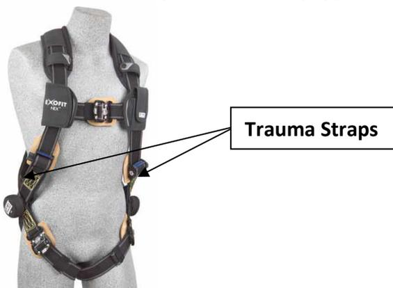
these may be taken out of their pouches and connected to establish a “platform” on which the worker’s feet can be placed for “standing” to relieve harness pressure. **NOTE: the worker must adjust the length of the trauma straps to accommodate his/her height after donning the harness and prior to beginning the work.**
